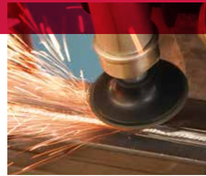
Blending disc smoothing weld seams.
