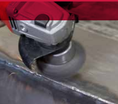
Knot wire cup brush removing heat discoloration.
