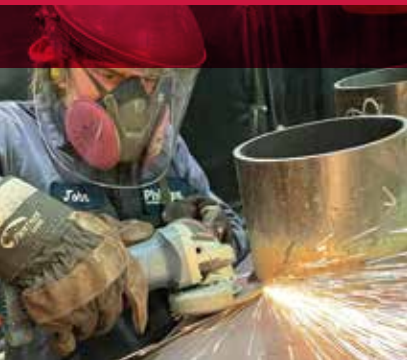
Weld blending on a stainless pressure tank with a Tiger Ceramic grinding wheel.
