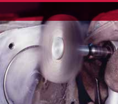
Removing carbon build-up from an engine.
